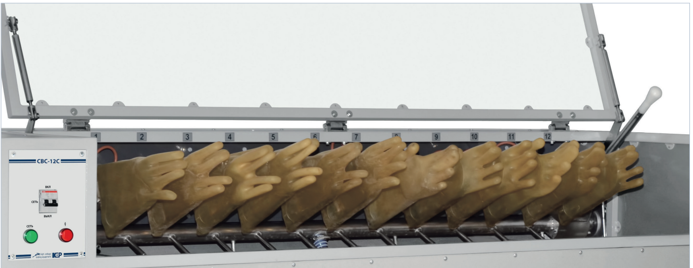
Testing dielectric gloves in CBC-12C bath
