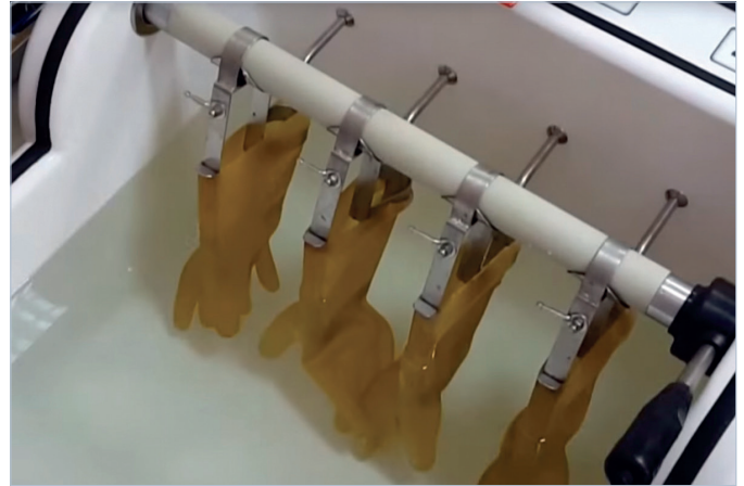
Testing dielectric gloves in CBC-C-series bath
