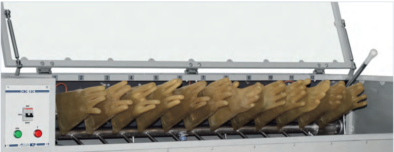
Testing dielectric gloves in CBC-12C bath
