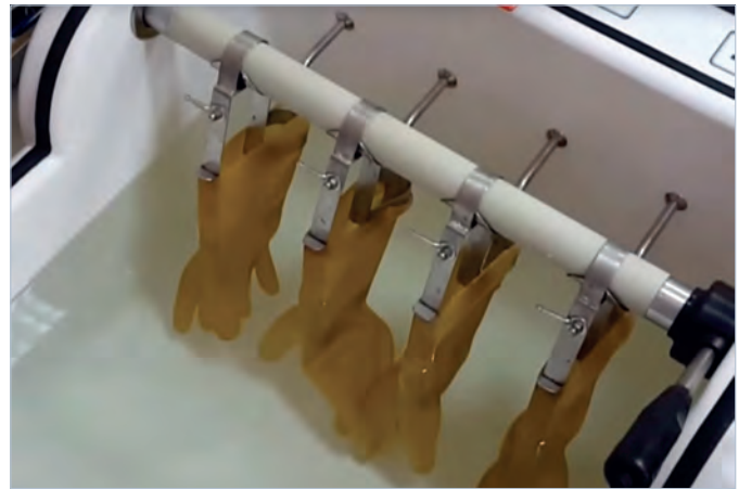
Testing dielectric gloves in CBC-C-series bath
